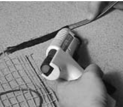
Either hot glue power lead into chiseled path . . .
